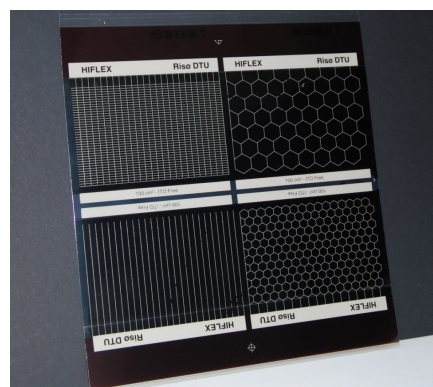
Silver screen printing for the serially connected devices (left) and An image of the monolithic cells prepared using four different silver grid patterns
