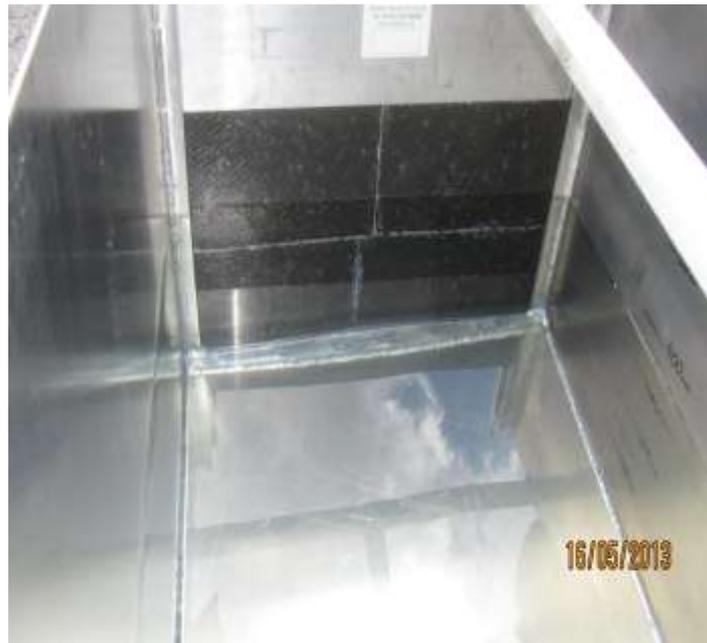
**Figure 8. Tank filled with water with the PRIME barrier in place to determine leakages or materials failure**
