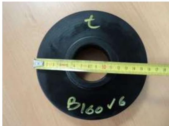
5. Elastic coupling. In this case, the rubber should also present a very good adhesion to the metallic parts.
