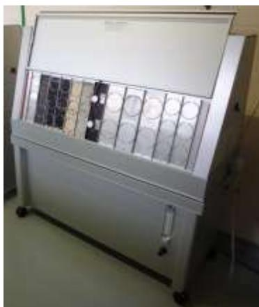
**Fig 3. UV cabinet according to EOTA (European Organisation for Technical Approvals) Technical Report which specifies exposure procedures for artificial weathering using EN ISO 4892**
