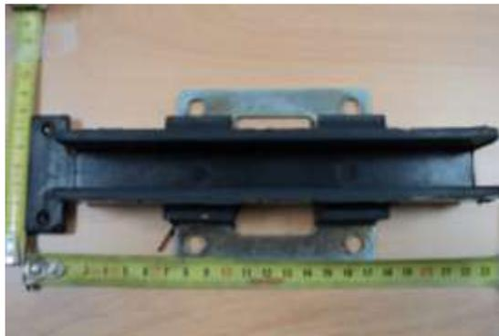
2. Draught excluder. The most important peculiarity of this piece is its reduced thickness, compared with the other two dimensions. In this case, the rubber should flow well enough when closing the mould, to fill it completely. Otherwise, air bubbles or lack of material could be observed in certain areas of the final product.
