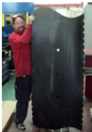
3. Bellows. In this case, the main particularity of the piece is its wavy shape, what makes the extraction from the mould a critical process. The rubber shouldn't present fragility when still hot, otherwise extracting the piece from the mould without harming the piece would be impossible.
