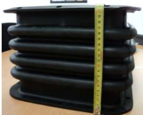
4. Elastic support. In this case, the main issue in the vulcanization process is that the rubber of inside the piece has to vulcanize completely.
